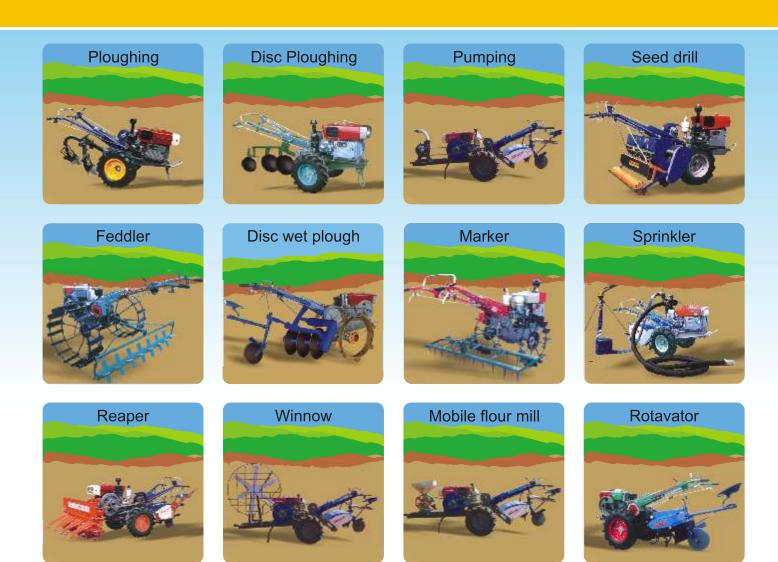
Power Tiller has the following equipment attached to for your advantage and profits. Plougher (dry & wet) used for alternating of soil at a depth of 12" by interchangeable double plough.
